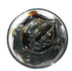
The multipurpose antifriction waterproof lithiumbased grease. Designed for use in friction units operating at temperatures from -20 °C to + 110 °C. Do not discharge into drains, soil and water
