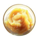
The multipurpose antifriction waterproof lithiumbased grease is made on the basis of highly refined mineral oils. Contains corrosion and oxidation inhibitors. Designed for use in friction units operating at temperatures from -40 °C to +120 °C. Do not discharge into drains, soil and water
